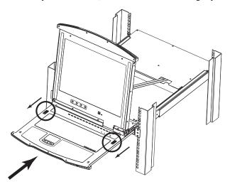
2. Let go of the catches. Using the front handle, push the keyboard module all the way in until it clicks into place.
